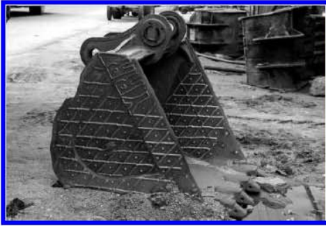
Figure 3 (above left) A simple strengthening would not have called for the care this backhoe bucket shows in its design of welded bracing, Rajasthan.
