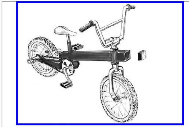
Kid's sheet-metal bike (Courtesy Interdesign 2005 Bicycle Group/ William (Morafo, Giovanni Toldo, and Martin Boshoff)
