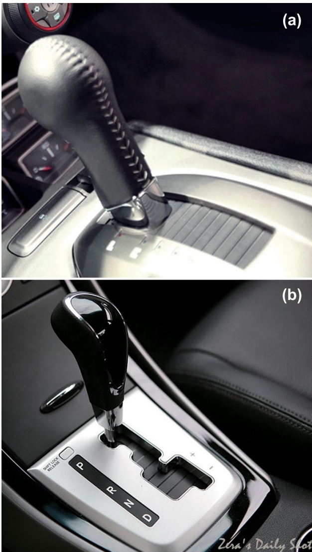
Figure 2. (a) I-shaped gate panel (Chevrolet Camaro, 2010) and (b) Steppgate-shaped gate panel (Hyundai Avante, 2010) [Photography by Zera with permission of Zera’s Daily Shot Blog]
