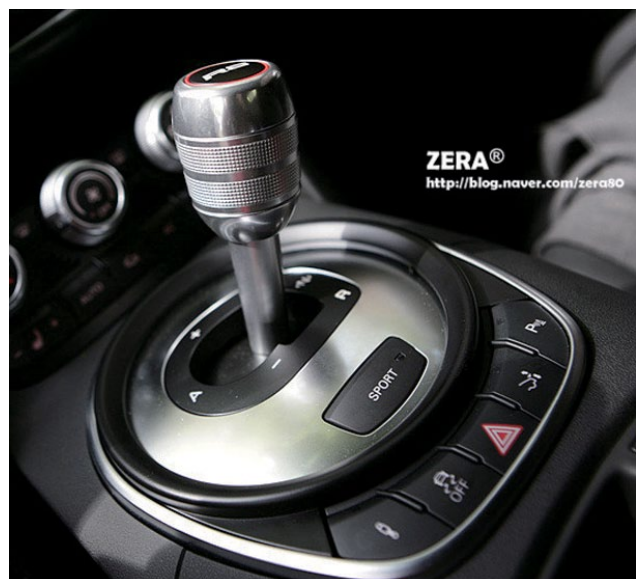
Figure 4. A shift panel design of Audi R8 that differentiates the movement range value. [Photography by Zera with permission of Zera’s Daily Shot Blog]
