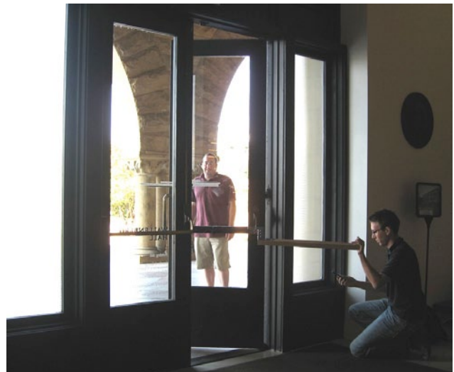
Figure 1. Wizard of Oz setup. A hidden door operator uses a mechanical armature to gesture the door.
