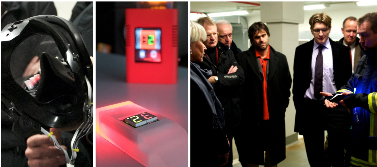
Figure 13. Navigation system in-mask display (left), beacon and handheld device (center), and firefighter explaining the system to stakeholders (right).
