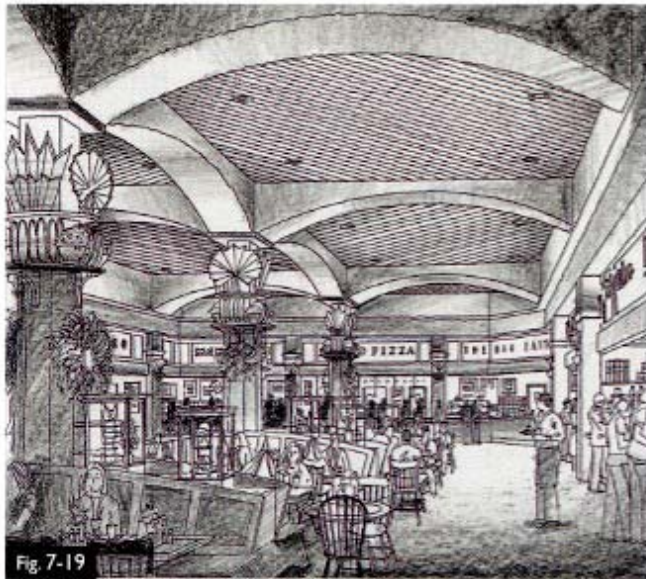
Fig. 7-19 The value study shown at the top is a 5" x 6" photocopy reduction of the line drawing. Note how the main part of the view appears brighter because of the darkened foreground.
