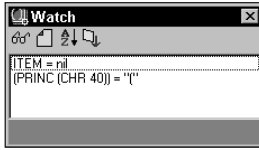
Figure 36-4: The Watch window shows an expression and a variable, and displays their values.
