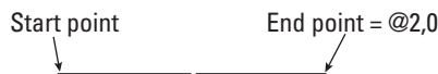
Figure 4-4: A line whose start point could be anywhere and whose endpoint is specified with the relative point @2,0 is a horizontal line two units long.
