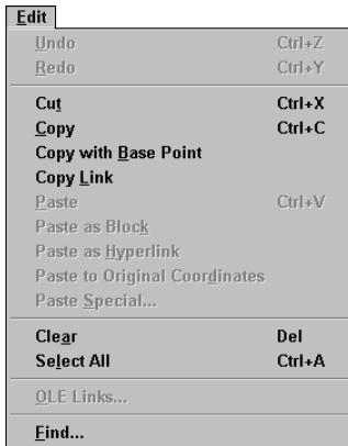
Figure 33-6: The Edit menu. Compare it to the menu code and look for the dividing lines and the underscored letters.
