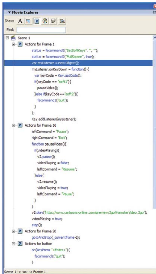
Figure 7.7 The movie explorer window showing all the action script to run a video player on your mobile
