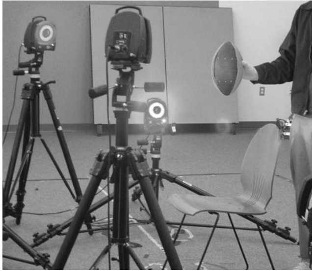
Figure 10.4 Checking camera setup with a marked football
