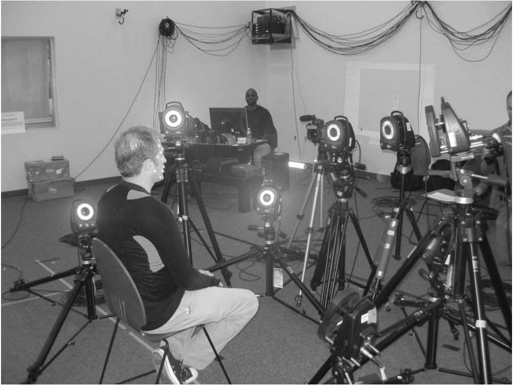
Figure 10.1 Camera setting for facial capture
