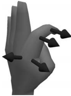
Figure 9.5 Two DOF at MCP and one DOF at joints between phalanges
