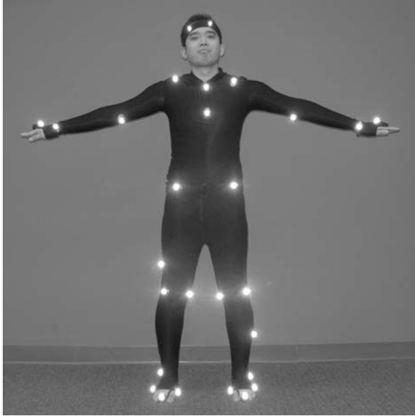
Figure 3.3 Subject with markers in a T-pose
