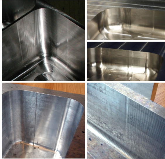
Fig. 1. Typical surface artifacts on milled surfaces. Top left: Marks resulting from changes of feed velocity. Top right: Chatter marks before and in corners. Bottom left: Artifact resulting from change of feed direction. Bottom Right: High roughness because of chatter marks.
