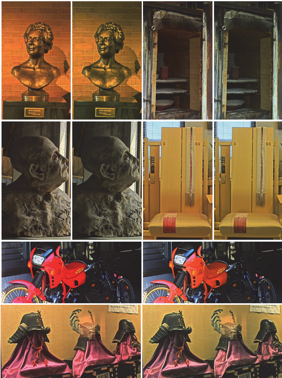
Fig. 24. Examples of the proposed mesopic filters. The leftmost image of each image set is without the filter; the rightmost is the varying filter. For these images, either the global or the local mesopic filter produces very similar results because there are no strong light intensities in the images, which makes the local averages to be somewhat close to the global average.
