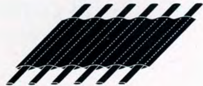
Single lamination showing primary fibres only.
