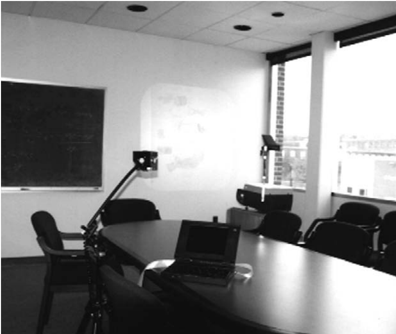
3.4. The cubic illumination meter in use in a small conference room where it is located at head height. It is controlled from the laptop computer
