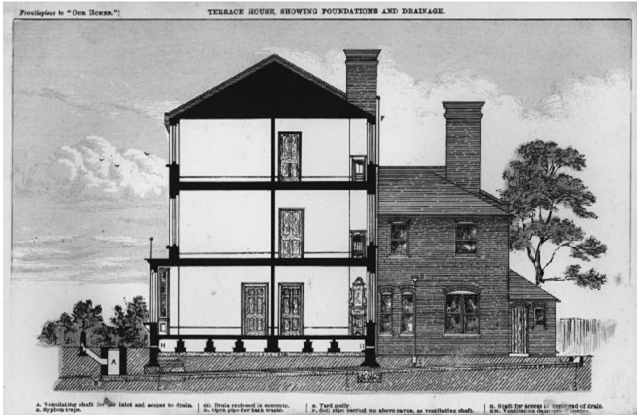
Figure 119 Terraced house, showing foundations and drainage.
