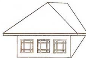
Dormer window vents attic space
