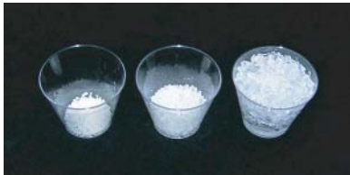
Polyacrylamide polymer crystals with a strong affinity for water swell to several hundred times their size in water, and then can revert back to their original size on drying
