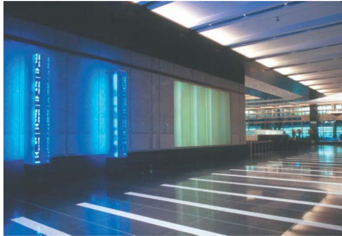
▲ Figure 7-8 Fiber-optics, dichroic glasses and LEDs were used by James Carpenter Design Associates in this lobby installation for Bear Stearns in New York. The green zone is produced with fiber-optics and dichroic glass, it serves as a soft contrast to the moving blue LED information screens. (James Carpenter)
