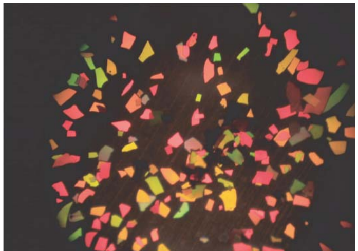
▲ Figure 5-17 Wireless sensor network. Top image shows prototype for a distributed sensor pod (NASA JPL). Bottom image shows 'smart dust' that functions as chemical sensors at the nano-scale level (Frederique Cunin, UCSD)
