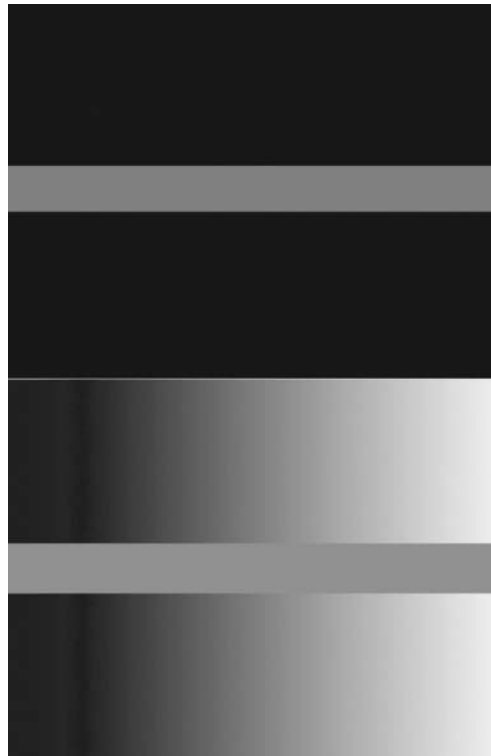
▲ Figure 3-16 Gray bar sequence. The center bars in both images have identical luminances, only the background is different. (Image courtesy of John An)
