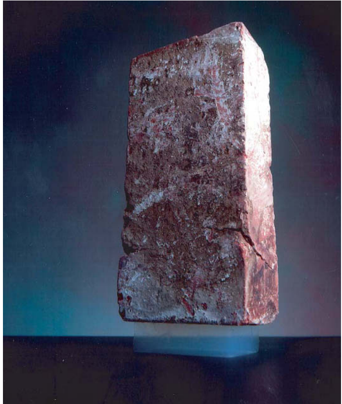
▲ Figure 1-4 Aerogel has a density only three times that of air, but it can support significant weights and is a superb insulator. Aerogels were discovered in 1931 but were not explored until the 1970s. (NASA)
