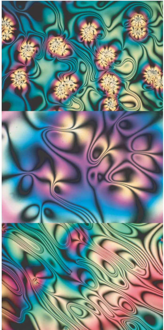
▲ Figure 4-9 Progressive phase change of nematic liquid crystal films (the typical thermotropic liquid crystal similar to what is used in LCDs). (Images courtesy of Oleg D. Lavrentovich of the Liquid Crystal Institute, Kent State University)
