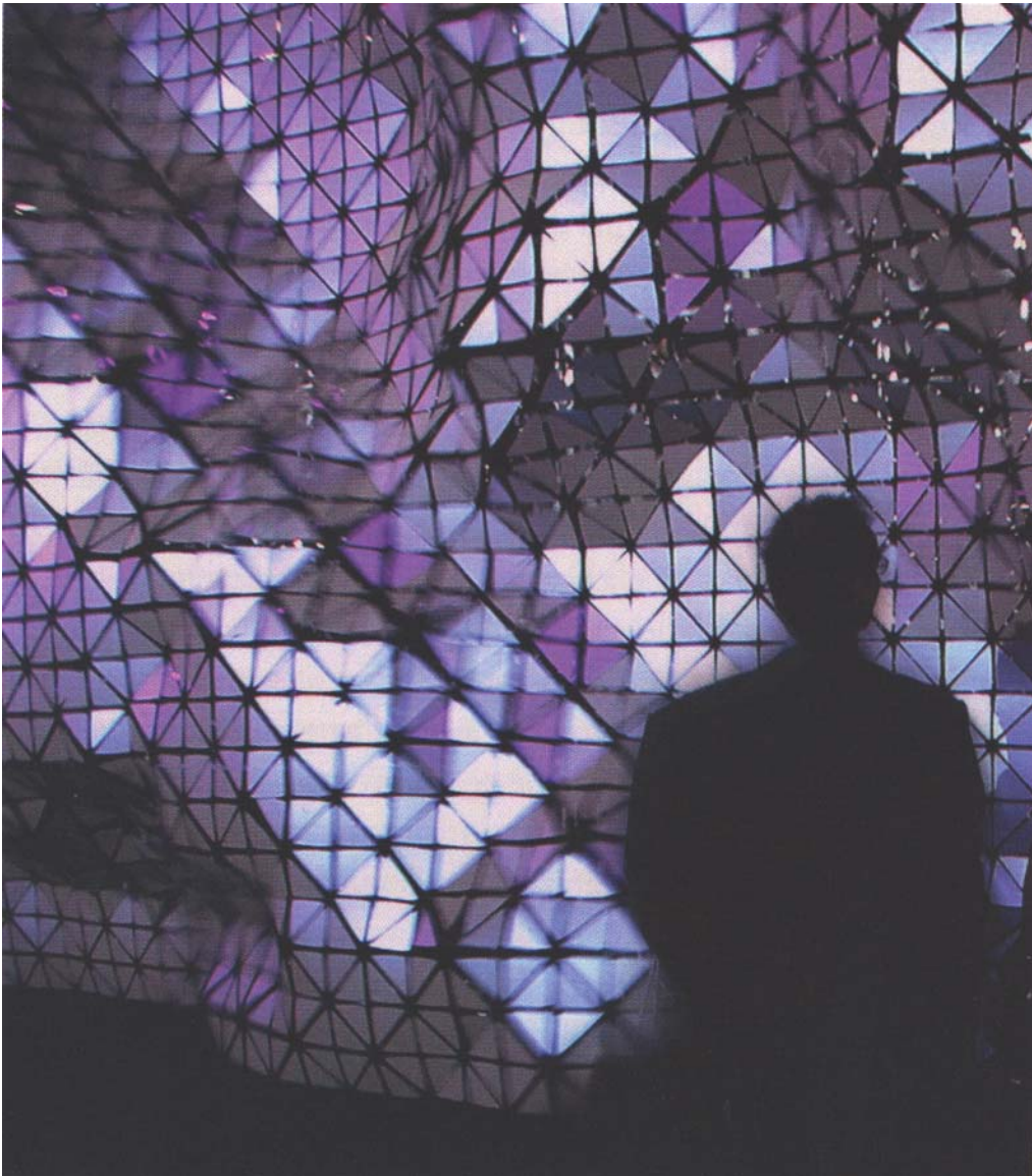
▲ Figure 5-4 'Hyposurface' installation combines position sensors with conventional actuators to create a responsive surface. Images courtesy of Marc Goulthorpe and DeCOI Architects
