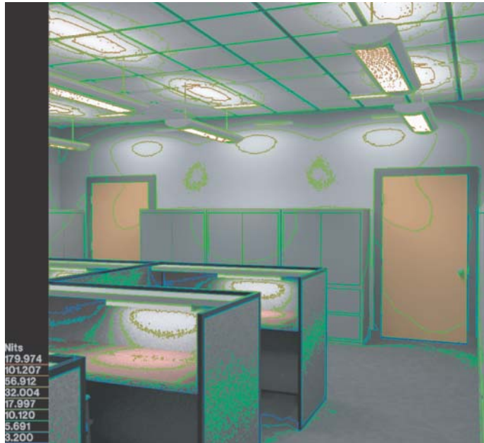
▲ Figure 9-3 Lighting simulation of interior office space using Radiance software. The contours illustrate the large variability that occurs in typical spaces. Simulation courtesy of John An.
