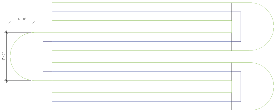
FIGURE 4.31 Modified ramp with curved boundary
