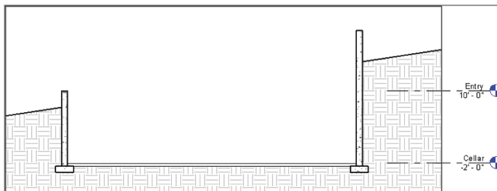
FIGURE 13.9 This section view illustrates how the building pad adjusts the extents of the topographic surface.
