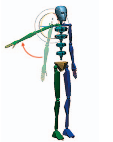
Rotating an arm or leg joint manipulates the joints by using forward kinematics.
