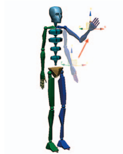
Moving a hand or foot manipulates the joints by using inverse kinematics.
