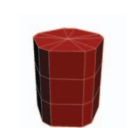
Gengon A cylindrical shape with user-defined fillets between the major sections.
