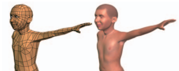
The high-resolution mesh (right) is manipulated by the low-resolution mesh.
