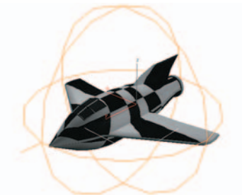
Spherical Maps the image to a sphere
