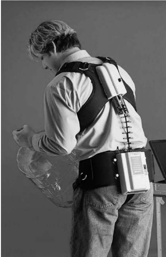
Figure 11.4 A lumbar motion monitor (LMM) worn by a worker can document worker exposure to dynamic work conditions. This information is used as part of the input to the risk model described in Fig. 11.3.
