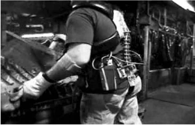
Figure 7.2 LMM used to collect information about kinematic exposure in industrial environments.
