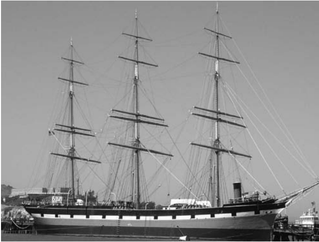
Figure 3.7 Support for a tall structure such as a mast is most efficiently provided by guy wires called stays and shrouds on a sailing ship. In a similar fashion, spine support is provided by the muscles and ligaments that run the length of the spine.
