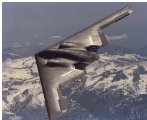
Fig. 3. The B2 spirit bomber, a reintroduction of an old idea, but this time with feasible flight control characteristics.
