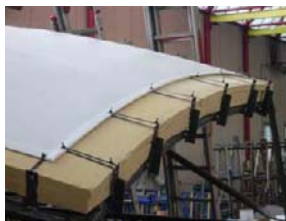
Fig. 21. First prototype with a stressed membrane.
