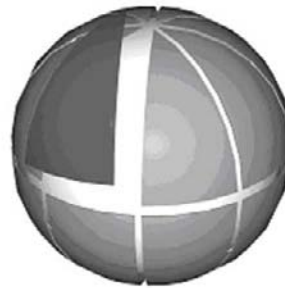
Fig. 6. Schematic drawing of the proposed division: 2 x 8 spherical segments in GRP.
