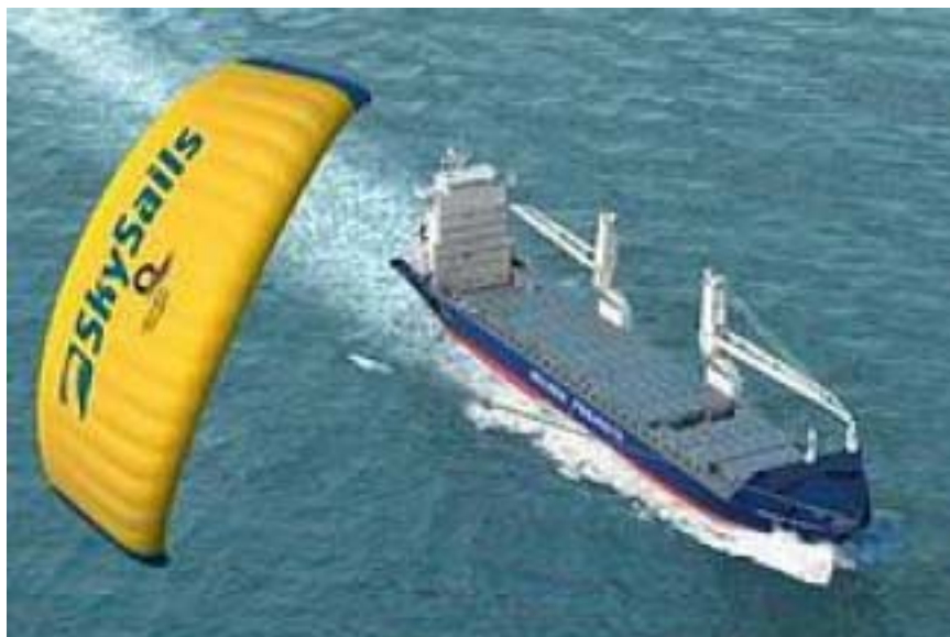
Fig 11. Applying a kite to a ship (source: sky sails, Germany)
