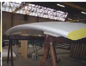
Fig. 23. Fourth prototype, a prefab sandwich construction.
