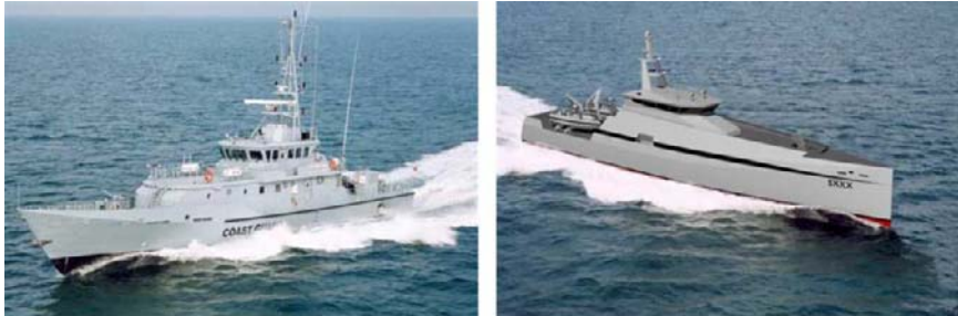
Fig. 6. Enlarged Ship concept (left) and Axe Bow (right) (by Damen Shipyards)
