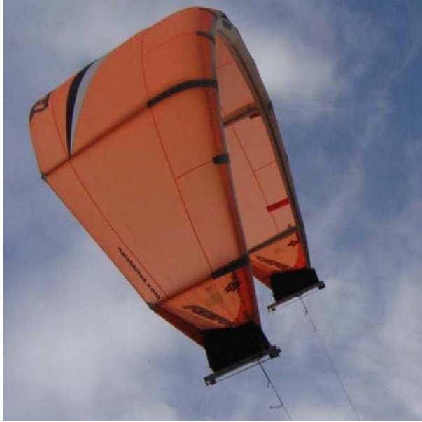
Fig. 8. Surf kite control by two wires only (source: Bas Lansdorp, Richard Ruiterkamp)
