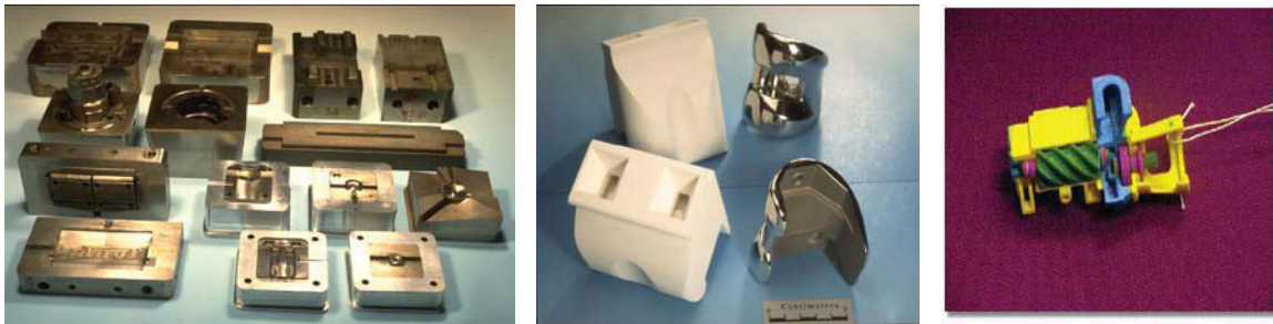
Fig. 5.20: Injection moulding tools made by 3D Printing; Ceramic mould made by 3D Printing and an orthopaedic knee casting poured into a similar mould; Colour-coded objects, such as this model of a compressor.
