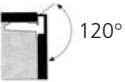
CONCEALED HINGE for standard cabinet lay-on doors. 120° opening angle with spring closing mecha- nism. Similar hinges for 100°, 107° and 170° opening
