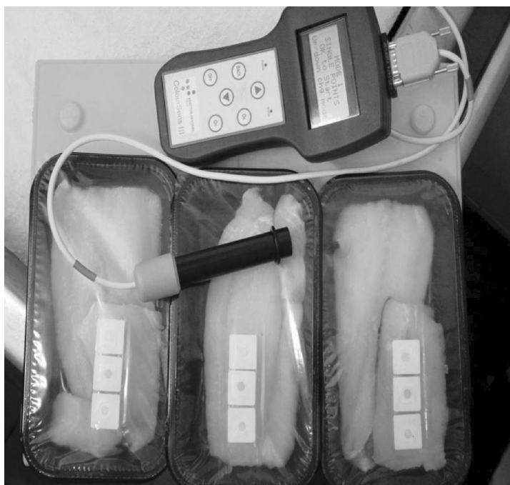
Figure 5.10 Examples of cod fillets packaged with three internal spoilage indicators (three different sensor formulations in each pack). The colorimeter and probe used for measuring the colour change are also shown.
