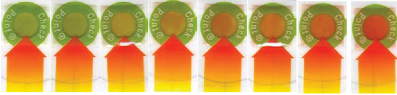
Figure 4.1 Response scale of enzymatic CheckPoint® TTI (Vitsab, Sweden).
