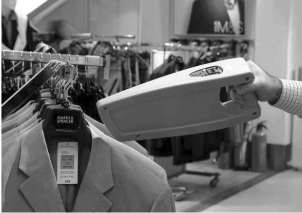
Figure 11.13 Hand-held scanner being used to scan jackets.
