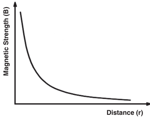
Figure 10.1 Attenuation of magnetic strength versus distance in near-field region.
