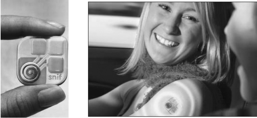
Figure 15.13 The SNIF fragrance device (left) can be placed anywhere on the body releasing perfume in accordance with the body conditions of the wearer (right). Reproduced with permission from PDD Ltd.
