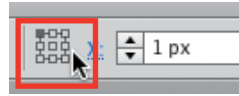
4.27 Change the origin point of an object with the reference point locator.
