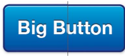
4.18 The left side of the button suffers from fuzzy-edge syndrome. The right side is crisp thanks to the pixel-snapping features in Illustrator CS5 and later.
