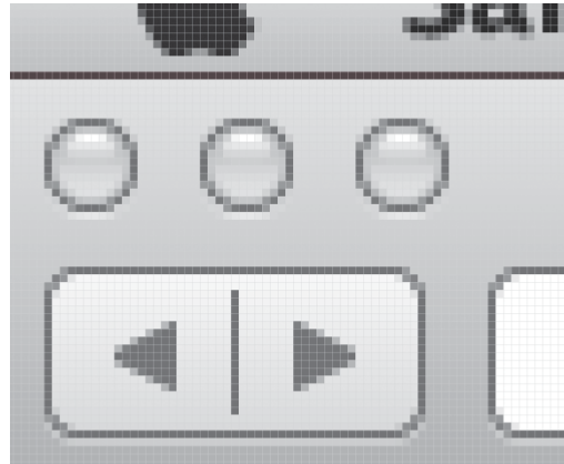
4.19 Pixel Preview mode allows you to see vectors as if they were bitmaps.
