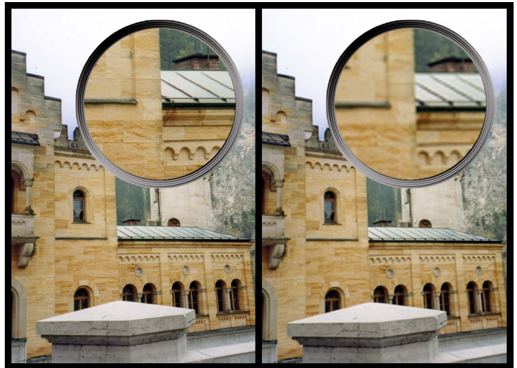
This photo was scanned at two different resolutions. The image on the left was scanned at 300 spi, and the image on the right was scanned at 72 spi. Examine the detailed enlargements to see the impact of different scanner settings.
