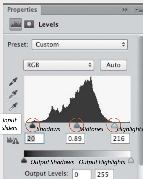
B The histogram in this Levels panel doesn’t extend all the way to the edges, an indication that the tonal range of the photo is narrow. To expand the range, we moved the Shadows and Highlights input sliders inward to align with the outer edges of the histogram, and moved the middle slider to the right to darken the midtones.
