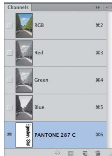
B Because our type shapes are now in a spot color channel, our commercial printer will be able to create a special printing plate for them.
