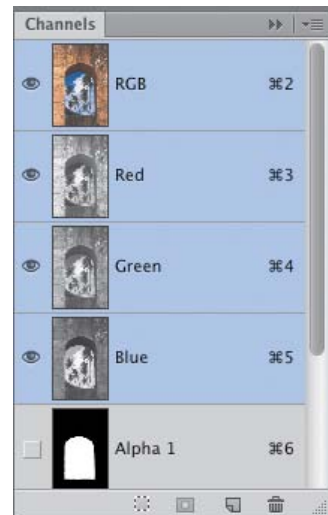
B ... then clicked the Save Selection as Channel button on the Channels panel. The Alpha 1 listing appeared.
