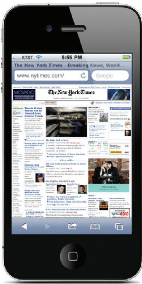
FIG 4.9: By default, Mobile Safari renders web content at 980px wide—even though its display is 320px wide when held in portrait mode.
