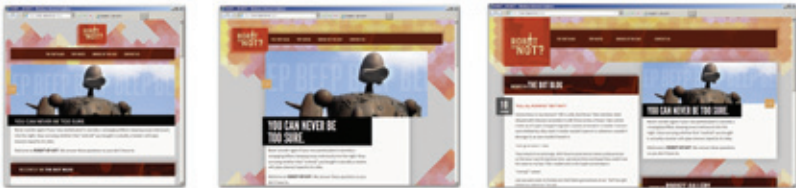
FIG 4.23: With our JavaScript patch in place, older browsers like IE now have some semblance of support for media queries.
