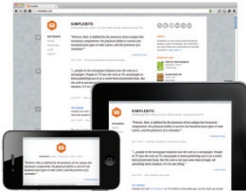
FIG 4.24: Dan Cederholm, the web designer's web designer, decided to set a max-width of 960 pixels on his newly responsive redesign. And you know what? It works.
