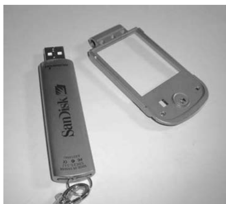
FIGURE 17.18 Photo of commercially available parts made of injection-molded metallic glass (SanDisk Cruiser® Titanium 512 MB USB memory stick and Liquidmetal® Technologies cell phone case).
