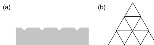
FIGURE 9.16 Graphoepitaxy. Graphoepitaxy allows for the growth of a single crystal layer atop an amorphous layer. Registration is achieved by patterning of the amorphous layer. The cross section of a patterned amorphous layer is shown in (a). A sixfold symmetric pattern, like that required for graphoepitaxially grown (111) silicon is shown in (b).
