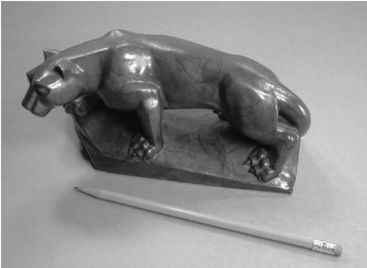
FIGURE 25.5 A slurry cast bronze statue formed using a wax-polymer binder, bronze powder, and rubber tooling. After the slurry was cast and cooled, the shape was placed in a furnace and slowly heated to burn out the binder and sinter the particles. This technology is ideal for smaller production quantities, such as encountered in the art field.
