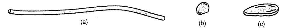
FIGURE 9.1 Possible physical shapes of imbedded phases in composite materials: (a) fiber, (b) particle, and (c) flake.
