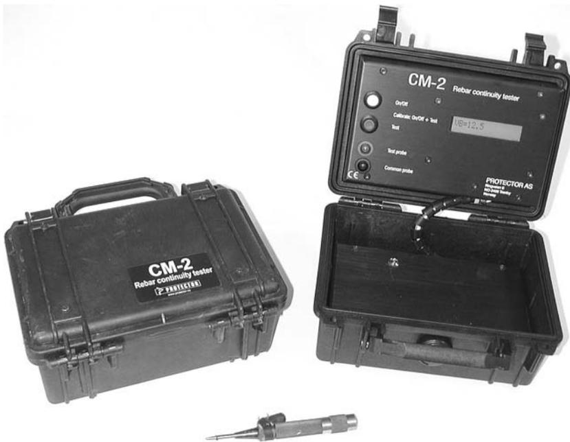
*Figure 8.13* Equipment for control of electrical continuity within the reinforcement system (source: Protector (2008)).
