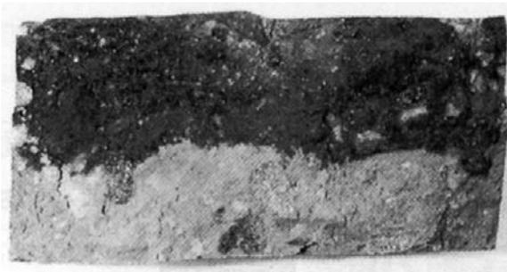
*Figure 8.5* Observed depth of chloride penetration on the split concrete surface after a spraying of the surface with a standard  $\text{AgNO}_3$  solution.
