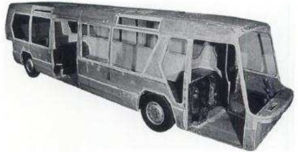
Above: Lightweight composite city bus weighing 999 kilograms.
