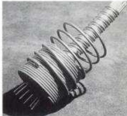
This kind of anchor at the end of a steel cable is difficult to translate into a solution for carbon cable anchoring.
