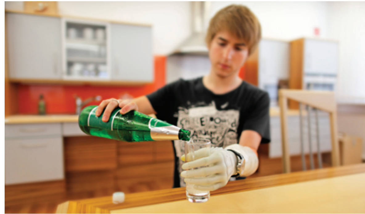
Figure 32: New prosthetics offer many advantages - gripping items such as a glass can be very difficult, if not impossible, with a traditional prosthetic hand. Photo courtesy of Otto Bock healthcare products GmbH
