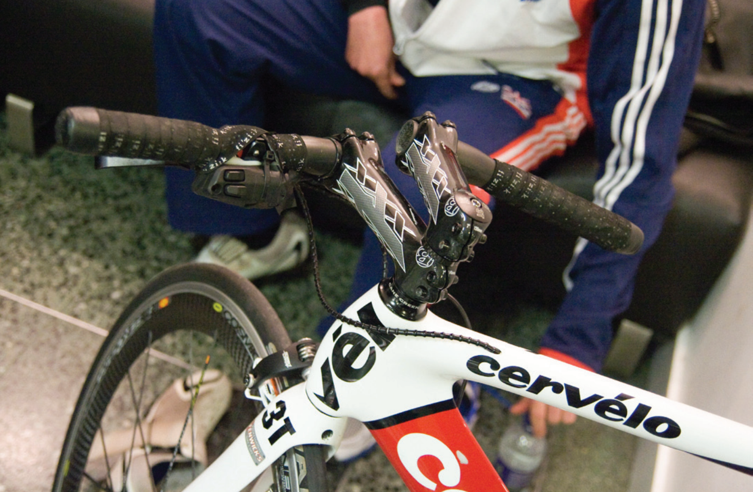
Figure 2: Custom bike handlebars and electronic gear shifters used by paratriathlete James Smith
