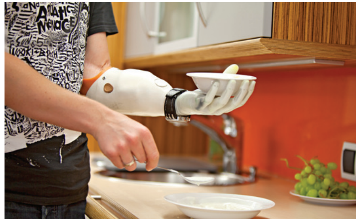
Figure 33: A further example of an action which is now possible but would not be using a traditional hook-based prosthetic hand. Photo courtesy of Otto Bock healthcare products GmbH
