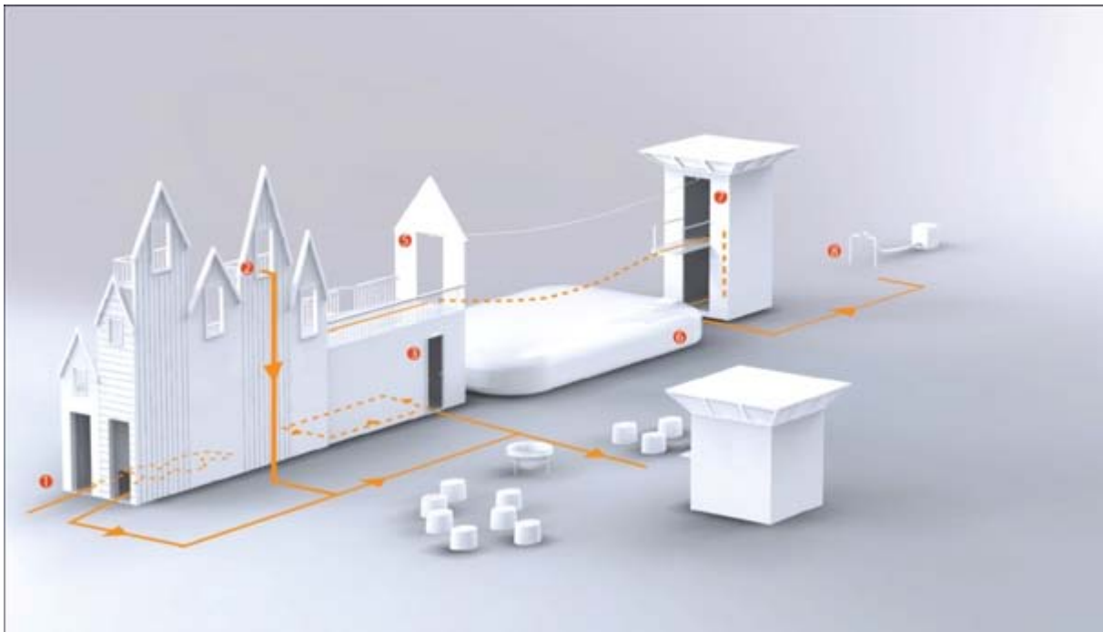
Fig. 13: The suggested training centre. This was a mobile unit designed to fit into a standard container size. Activities like testing escape ladders and ropes, jumping onto fire escape cushions and finding the way in smoke filled labyrinths are indicated. (Student: Heidi Borthne, 2009)
