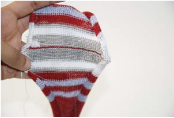
Figure 6. Opened view of reversed side of sleeve - Conductive yarn knitted in rows to form a location switch circuit.
