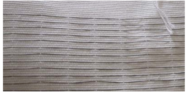
Figure 1 Sample of woven cotton with conductive threads on one side. The threads can serve as heating elements and thus change the color of a thermo chromatic pattern printed on the other side.
