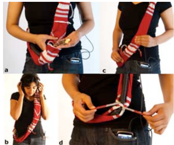
Figure 2: a) An opening that allows coins to be dropped into the sleeve. b) The sleeve is worn across one's shoulders. c) Rotating the sleeve moves the coins within. d) The movement of the coins can be obstructed by tying the string.
