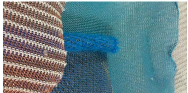
Figure 3 Three samples of textiles knitted with different strength of conductivity. Left: knitted copper with viscose. Center: knitted blue mohair with brass. Right: knitted turquoise cotton with stainless steel.
