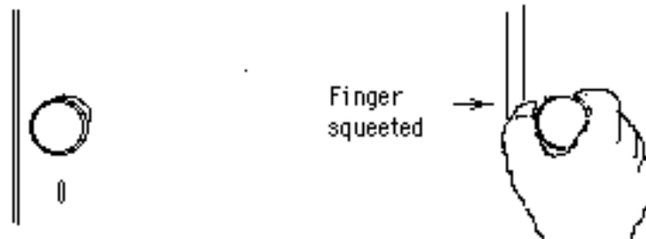
Figure 3.9-1: Door knob I: How to open it? The lock is under the knob, and it is not easy for human eyes to see the lock. Sometimes, finger got squeezed.
