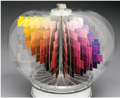
This is a set of calibrated color samples. Each is designed to be equally different from the adjacent sample, making it an example of a uniform color space . (From Science Museum/ Science and Society Picture Library, London.)
