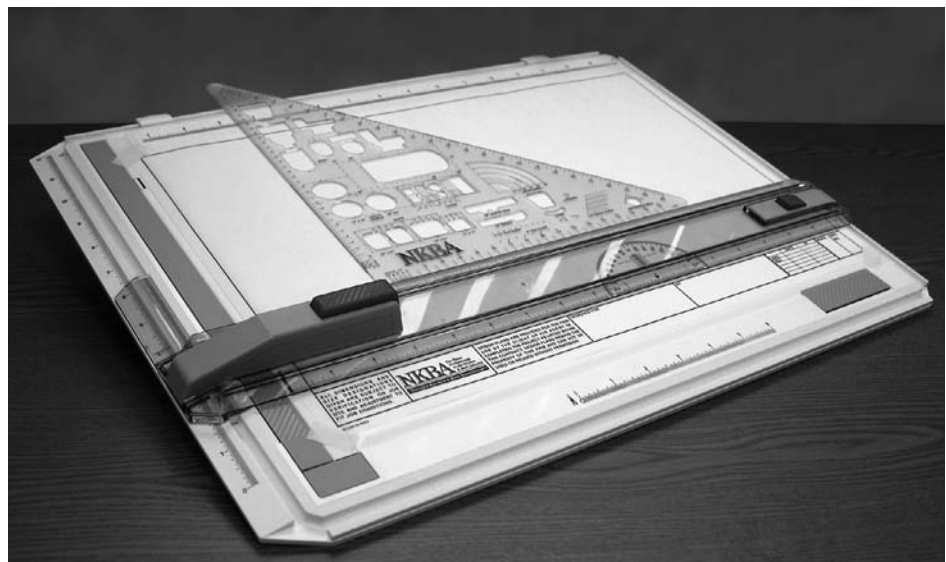
FIGURE 5.6 Align the sheet of vellum using your parallel bar or straightedge and one of the horizontal border lines.
