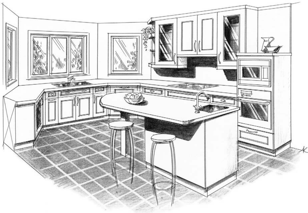
FIGURE 6.22 Shading a drawing using gray tones. Courtesy of Tony Hunt, CKD, CBD
