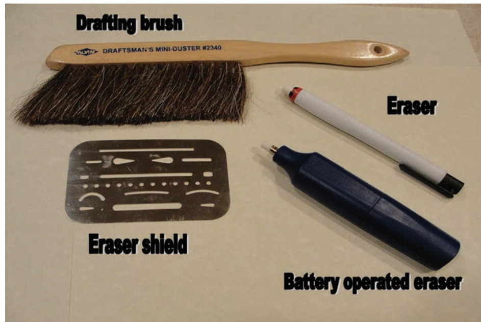
FIGURE 3.11 Two of many available erasers, eraser shield, and drafting brush. The eraser shield allows for precision erasing. Always use the drafting brush to brush off eraser crumbs and graphite.
