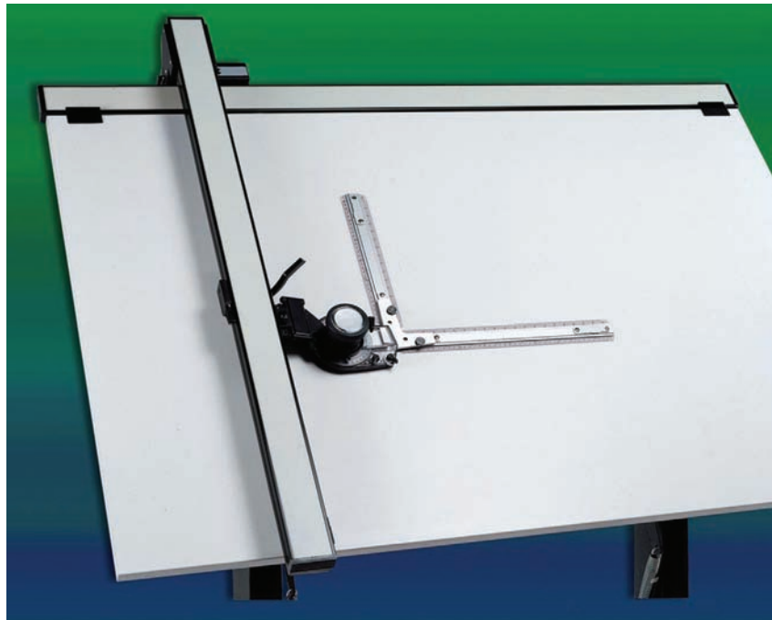
FIGURE 3.6 Drafting machine fastened to the drafting board. Can be left- or right-handed.
