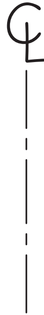
FIGURE 8.17 The centerline symbol used to show center points of all appliances, fixtures, etc.
