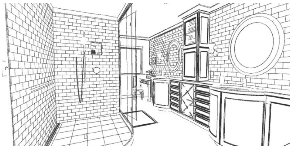
FIGURE 1.9 A perspective drawing provides a three-dimensional view of the space, showing depth. This drawing closely resembles how the human eye sees a space.
