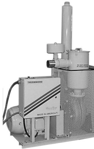
Turbine Vacuum Pump
