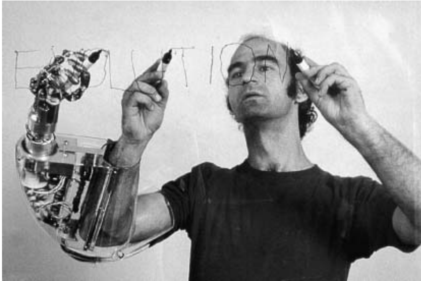
Figure 2.7 In Third Hand , Stelarc wrote single words with a third artificial hand strapped to one of his own, activated by the EMG signals of the abdominal and leg muscles, while the real arm was remote-controlled and jerked into action by two muscle stimulators.
