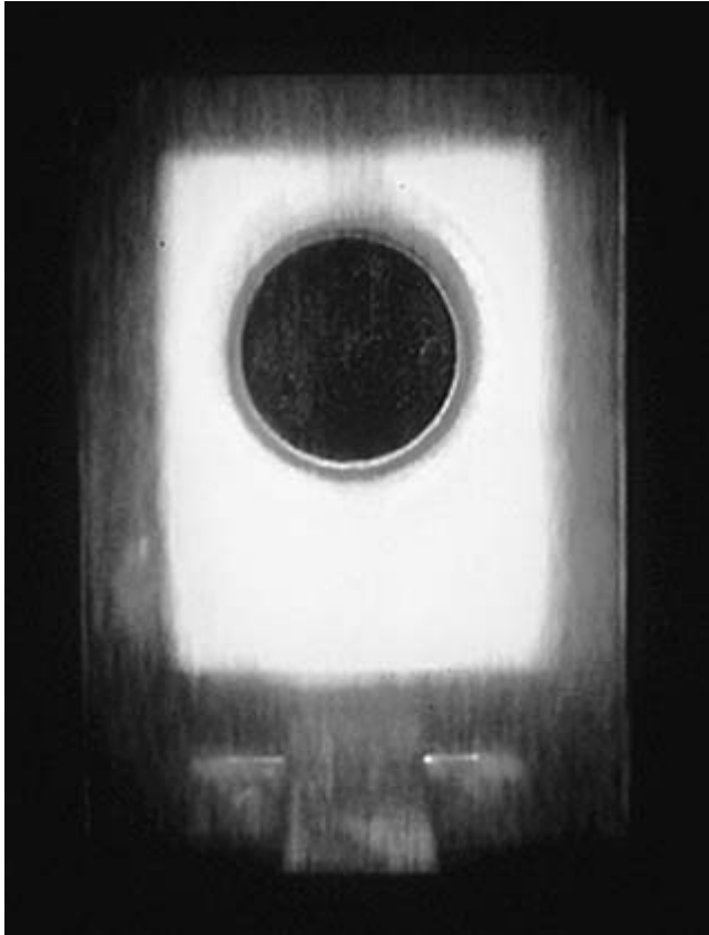
Figure 7.8 LCD screen encapsulated in fluorescent polycarbonate.
