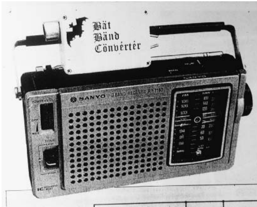
Figure 6.14 The Bat Band Converter from Everyday Practical Electronics is a parasitical device that allows you to “use your AM portable radio and this novel design to tune-in to the secret world of bats.”
