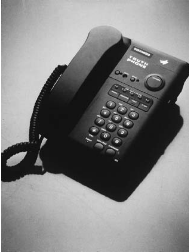
Figure 4.5 Truth Phone TM , by the Counter Spy Shop, is an example of an object embodying a pathological model of behavior. It combines a voice-stress analyzer and telephone, allowing the user to tell whether the person at the other end is lying.
