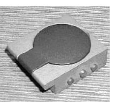
Fig. 15. An alarm clock. (Volume: 4x3x1 cm, weight: 400g)
