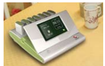
Fig. 5 The touchscreen panel with adjustable angles (0°~45°)
