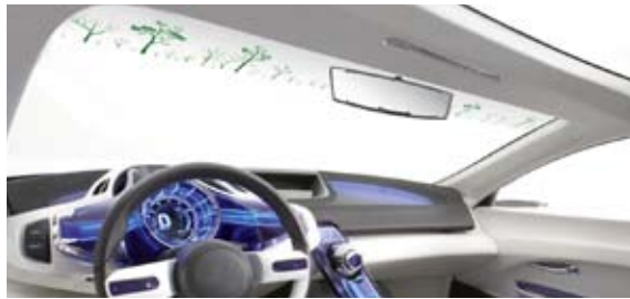
Fig. 3. A long strip of e-paper powered by sunlight provides a driver with feedback
