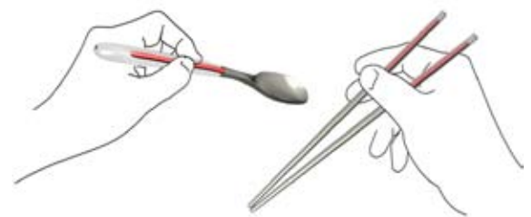
Fig. 1. Dining ware embedded with motion sensors
