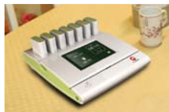
Fig. 3 One main server with seven portable pillboxes
