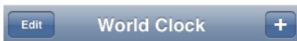
Figure 5-6 A navigation bar can contain controls that manage the content in the view
