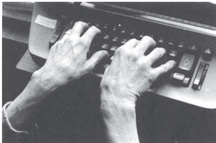
Figure 86 Position of wrists and hands operating a traditional keyboard. The parallel position to the rows requires an inward rotation of the forearms and wrists and a sideward twisting (lateral abduction) of the hands.
