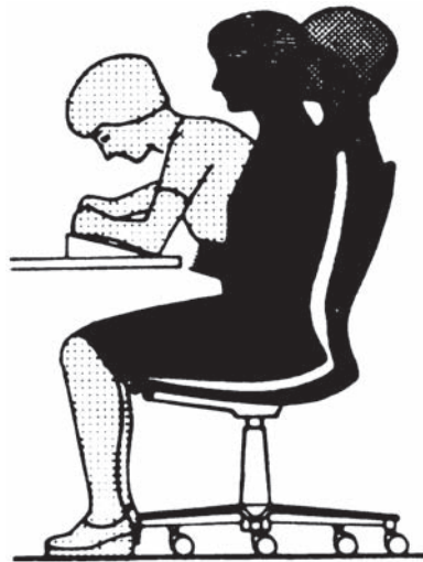
Figure 73 An office chair must be conceived for a forward as well as backward inclined sitting posture.
