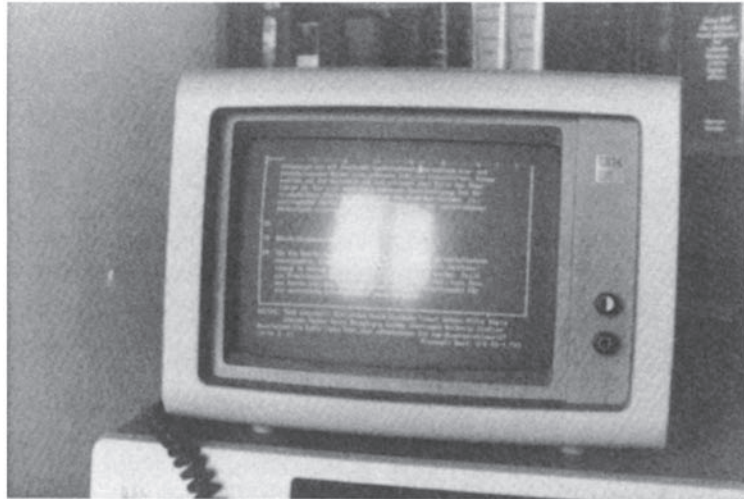
Figure 26 The reflected image of a window behind the back of the operator is superimposed on the screen text and disturbs reading.
