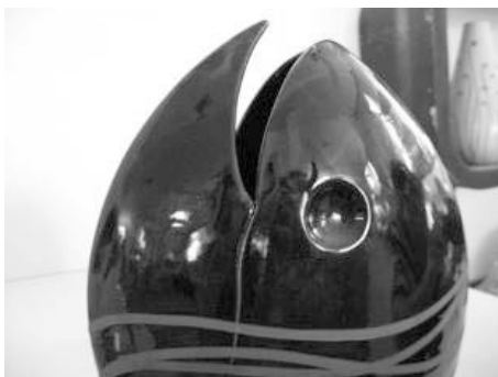
Before: sharp angle of mouth caused product to often cracking during firing
