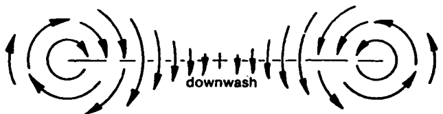
Fig. 5.4 The downwash behind a wing between the tip vortices
