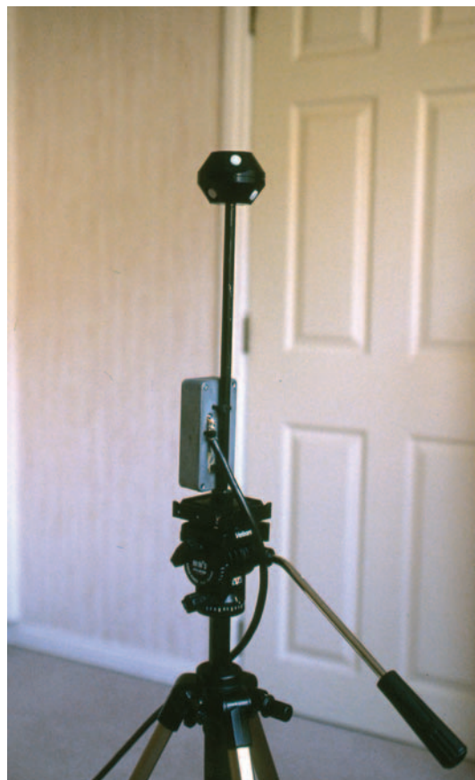
Figure 3.6: The vertical axis cubic illumination meter is mounted on a tripod and controlled from a laptop computer, which scans the six photodiode outputs and computes vector and symmetric illuminances on the x , y , and z axes
