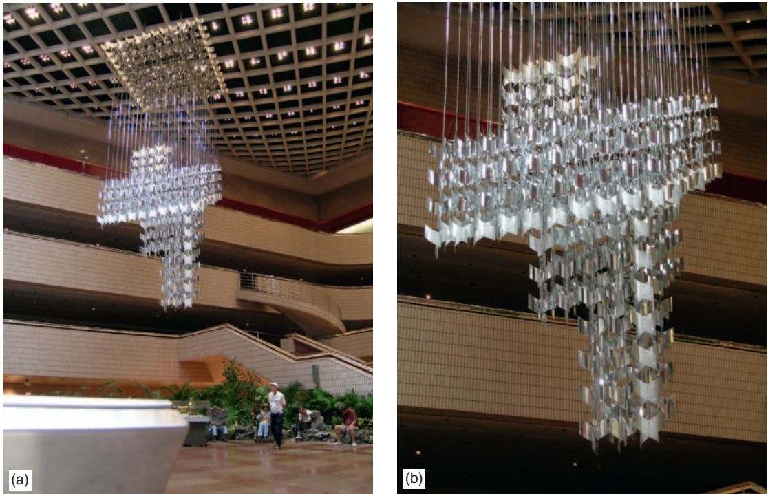
Figure 2.46: This eye-catching pendant (a) at the Hong Kong Cultural Centre appears to be a luminaire, but on close inspection (b) it is seen to be a specular metal sculpture lit by concealed spotlights
