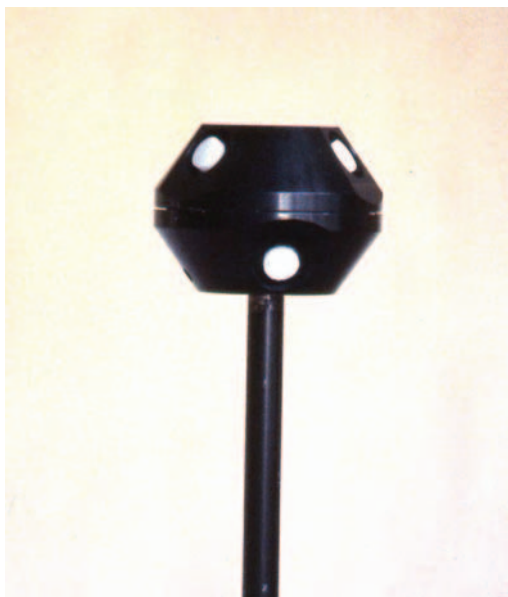
Figure 3.5: Vertical axis cubic illumination meter. Six silicon photodiodes are aligned on the faces of a cube tilted so that one long axis is vertical. The axes of the opposing pairs of photodiodes are designated u , v , and w
