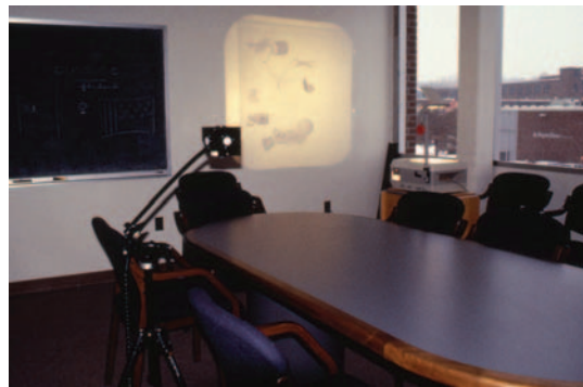
Figure 3.4: The cubic illumination meter in use in a small conference room where it is located at head height. It is controlled from the laptop computer
