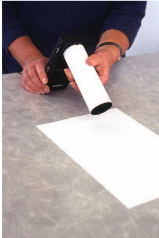
Figure 3.9: A reading for the patterned worktop material is compared with a sheet of white paper to obtain an estimate of reflectance
