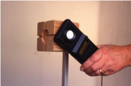
Figure 3.2: Measuring illuminances on the six faces of a cube
