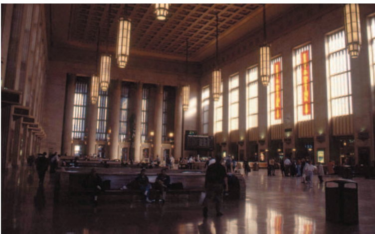
Figure 2.41: The renovated luminaires in this Philadelphia railway station are switched on all day, even though the daylight streaming in through the windows provides perfectly adequate illumination
