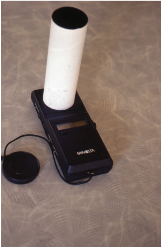
Figure 3.8: An illuminance meter adapted with a cardboard tube, internally sprayed matt black, for making relative luminance measurements
