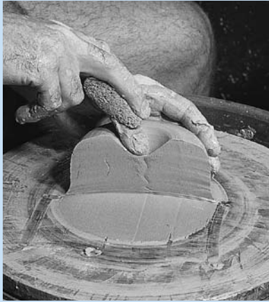
a. Cross sections of basic thrown form: Creating the dimple.
