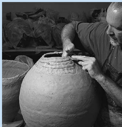
g. Smear additional coils inwards to reduce the opening.
