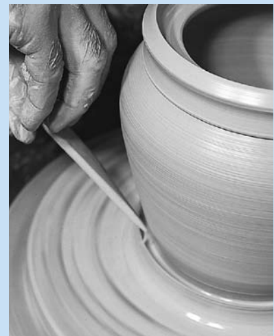
b. Dribble water along the knife to feed it into the cut.
