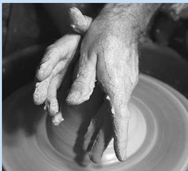
g. With continuing side pressure to prevent mushrooming, press clay back down.
