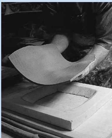
a. Using a foam slump mold: Drape a slab over the mold.
