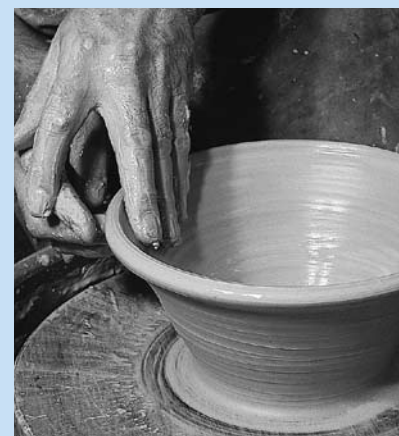
b. Lift repeatedly, maintaining straight walls.
