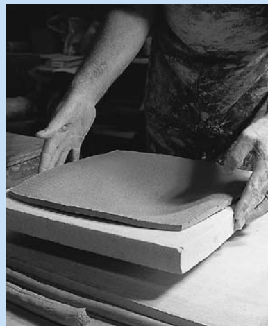
b. Gently drop the mold repeatedly to settle the slab into the mold.
