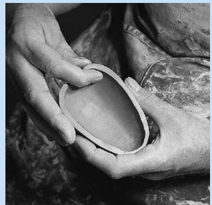
h. With a finger inside, smear the clay inwards to reduce the opening.
