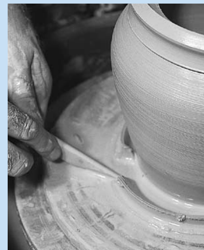
d. Stop the wheel, cut through the waste flange, and remove it from the pot.
