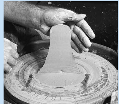
f. Cross section showing maximum rise, with heel of thumb poised to press clay back down.
