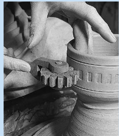
c. Using a wooden roulette.
