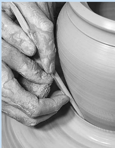
a. Trimming excess clay away from base of finished pot: Slice into the clay with a wooden knife.
