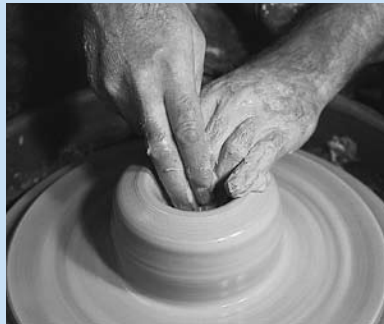
b. Penetrate the lump to create a V-shaped opening.
