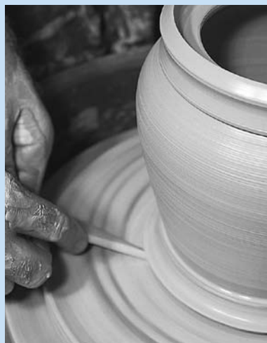
c. Slice horizontally under the waste flange with the wooden knife.
