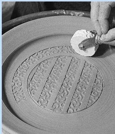
a. Using a bisque roulette on a plate.
