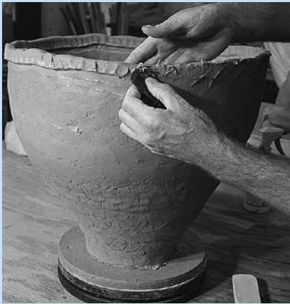
c. Smear the soft coil downwards inside and out over the stiffened edge.
