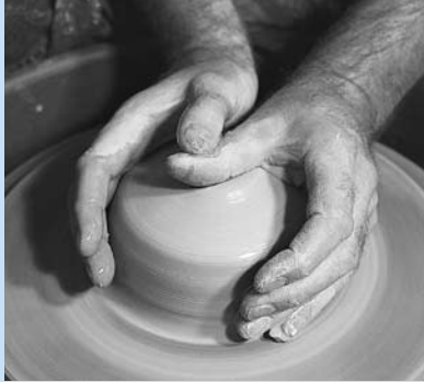
a. Centering and wheel wedging: Initially center the clay with firm side pressure.
