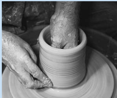
h. Begin second lift, pressing into the clay at the base.
