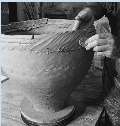
f. After every three or four courses, smear the coils together with diagonal strokes.
