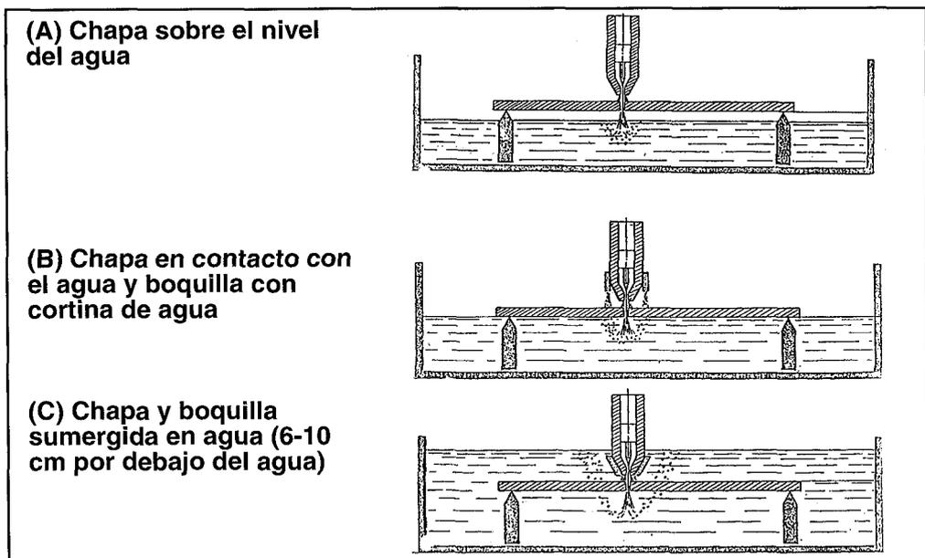
FIGURA 8.12: CORTE POR PLASMA CON MESA DE AGUA
