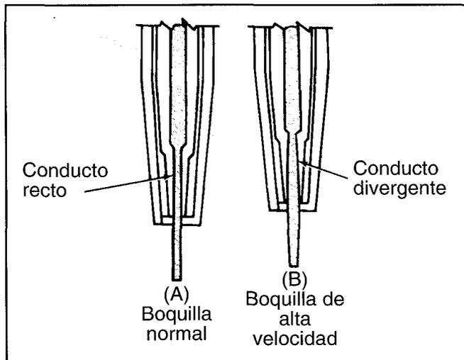
FIGURA 8.6: TIPOS DE BOQUILLA PARA OXICORTE
