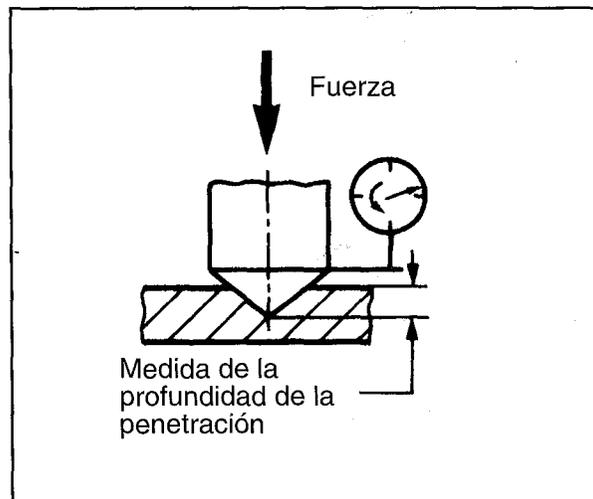
FIGURA 19.4: ENSAYO DE DUREZA ROCKWELL
