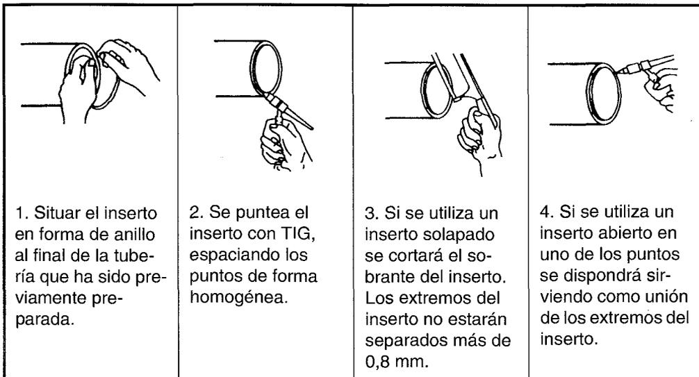
FIGURA 12.14 (C): PASOS A SEGUIR PARA SOLDAR TUBERÍA CON INSERTOS CLASE 1, 2, 3 Y 5
