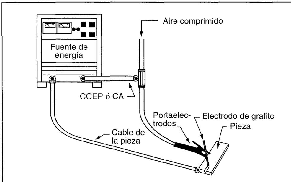
FIGURA 8.16: EQUIPO DEL PROCESO ARCO-AIRE
