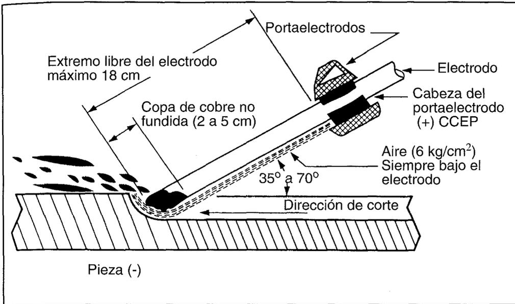
FIGURA 8.17: ELECTRODO PARA ARCO-AIRE
