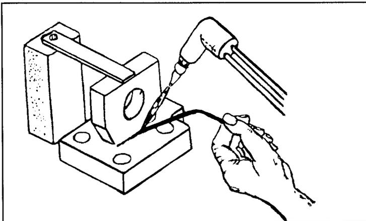
FIGURA 17.4: SOLDEO FUERTE O BLANDO CON SOPLETE
