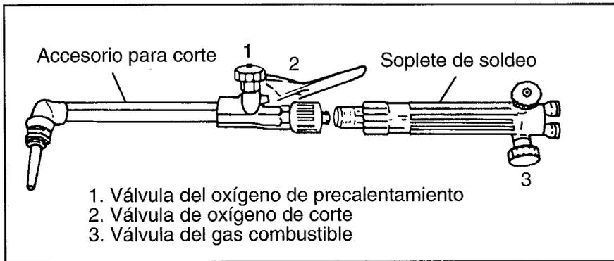
FIGURA 8.4: SOPLETE MANUAL COMPUESTO
