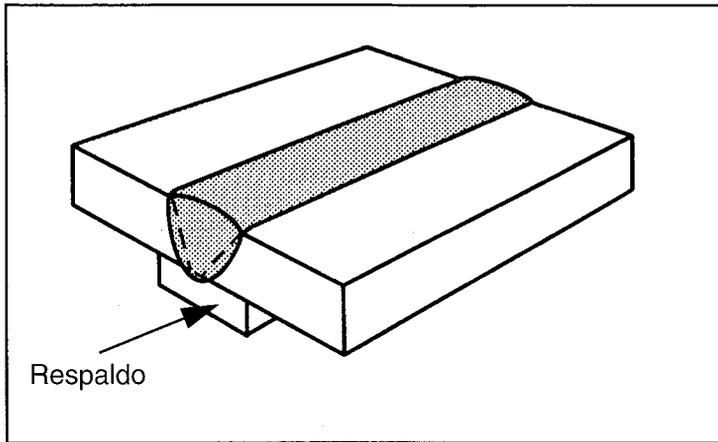
FIGURA 5.11: SOLDADURA CON RESPALDO
