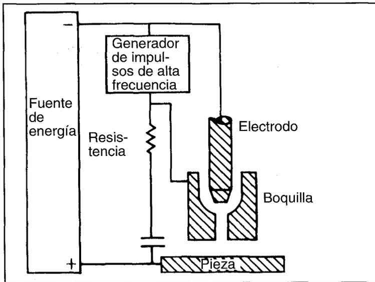
FIGURA 8.11: EQUIPO PARA EL CORTE POR PLASMA
