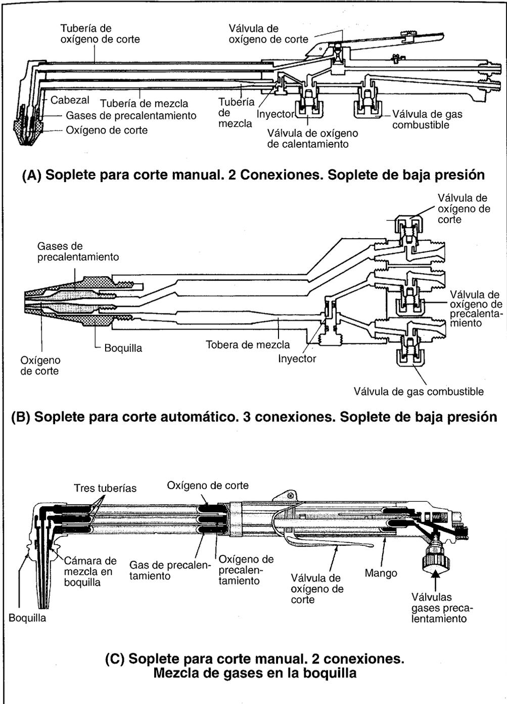
FIGURA 8.5: DIFERENTES TIPOS DE SOPLETES
