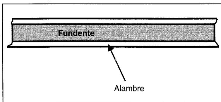
FIGURA 14.6: ELECTRODO-ALAMBRE TUBULAR
