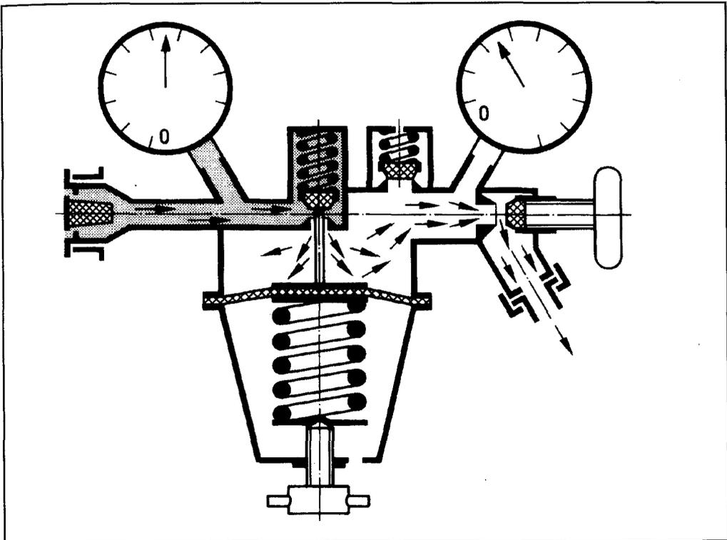
FIGURA 9.9: MANEJO DEL MANORREDUCTOR. APERTURA
