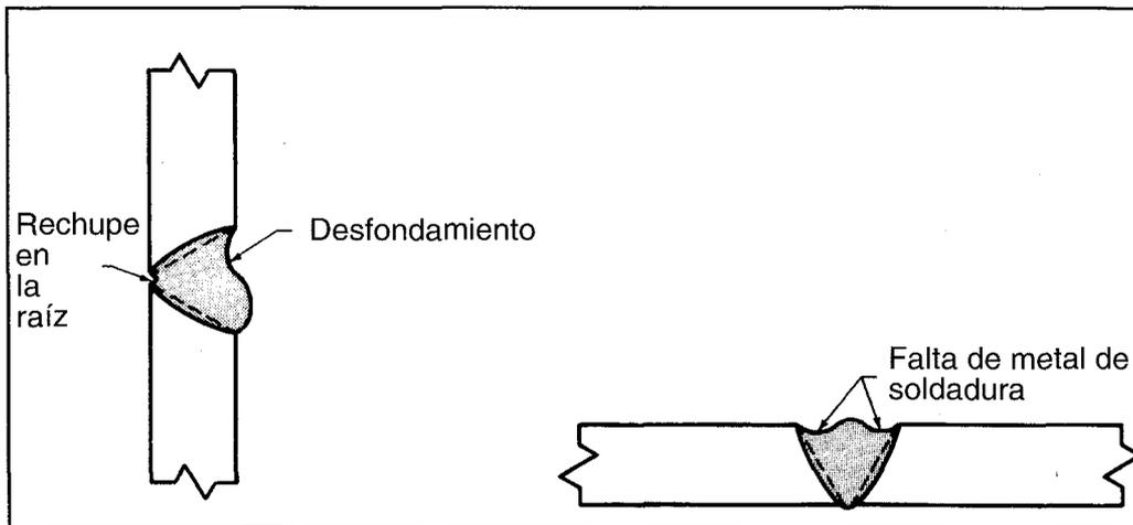
FIGURA 30.11: FALTA DE METAL DE SOLDADURA
