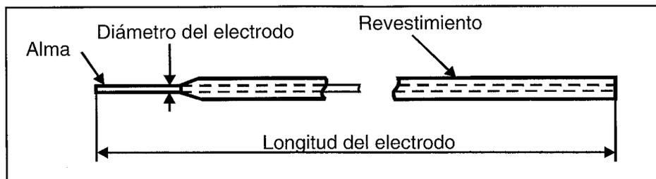
FIGURA 10.5: ELECTRODO REVESTIDO
