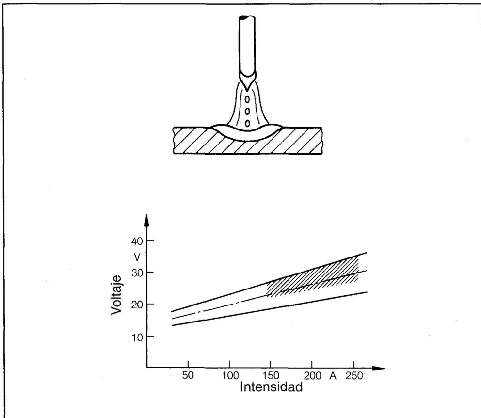
FIGURA 13.17: TRANSFERENCIA POR ARCO SPRAY
