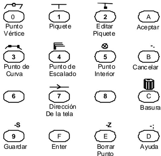
Figura 6-1d El cursor de 16 botones Numonics Accugrid A-90 XNT.
