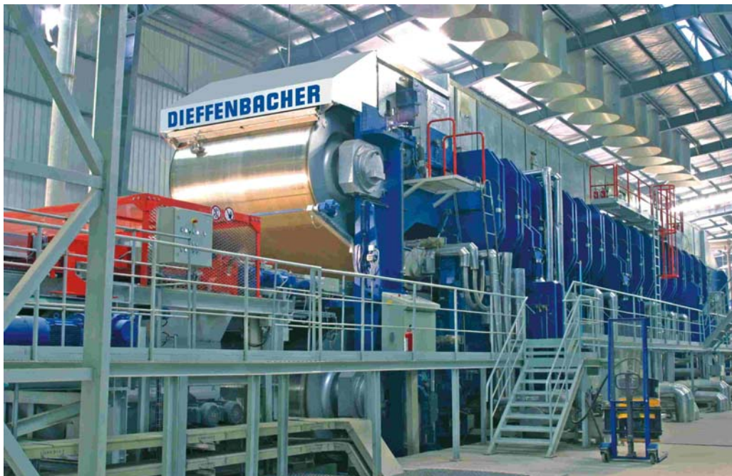
Figura 9. Prensa Conti Panel System (CPS) , (cortesía Dieffenbacher).
