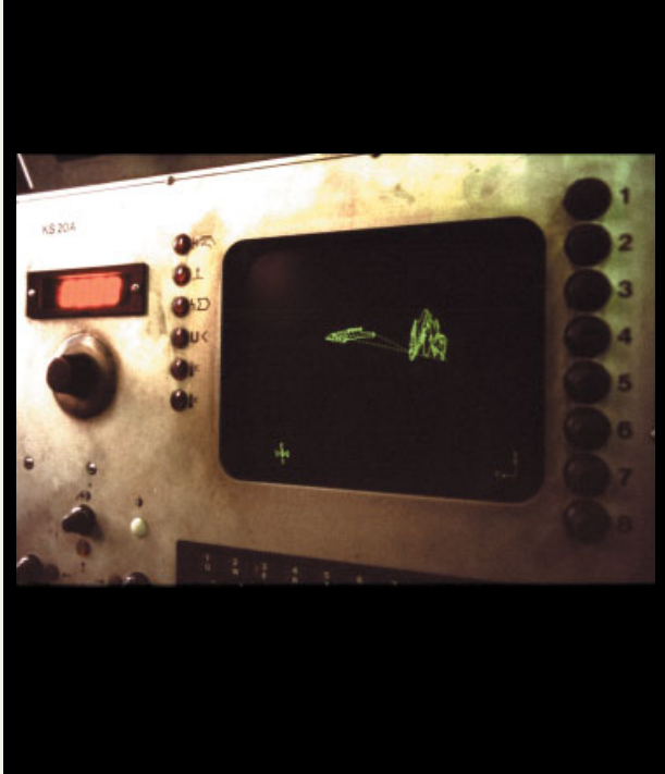
sixteen*[makers], Blusher project, Güsten, 2001 Components of the project awaiting digital fabrication momentarily appear on the CNC plasma-cutter's monitor; 45 minutes later, all 21 pieces were complete.
